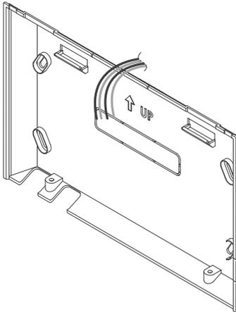
4. Connect the RS485 cable, which is located behind the AC Smart Premium, to the RS485 terminal.
